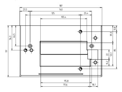
Adapter 74 111 0019 0 for Screw-less Mounting, (H = 56mm) on DIN-Meters
