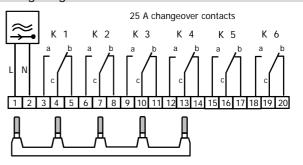
Phase link for connection of L with relay levers for K1-K4. Possibility to shorten for 1, 2 or 3 relays. The bare metal cut will be insulated by protection cap.
