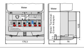
Adapter 4 111 2361 0 for Mounting on ZMB, ZMD...CT and ZMD...AT Meters, (H = 74mm)
