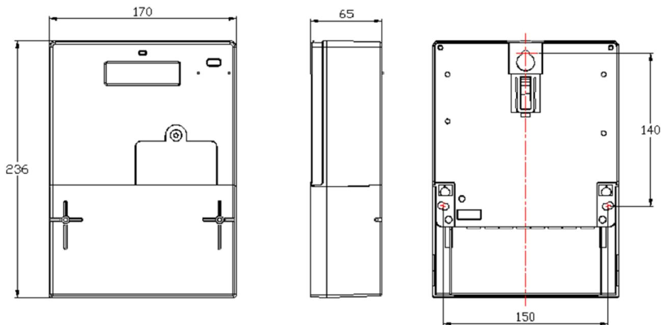
**Abmessungen Klemmen****E220-AM1D 60 A Direktanschluss**
